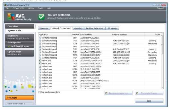
The **Network Connections** dialog contains a list of currently active connections. The list is divided into the following columns:
