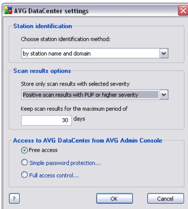
The **Station identification** section contains a drop down menu, where you can select how you wish to display stations within the current view section.
