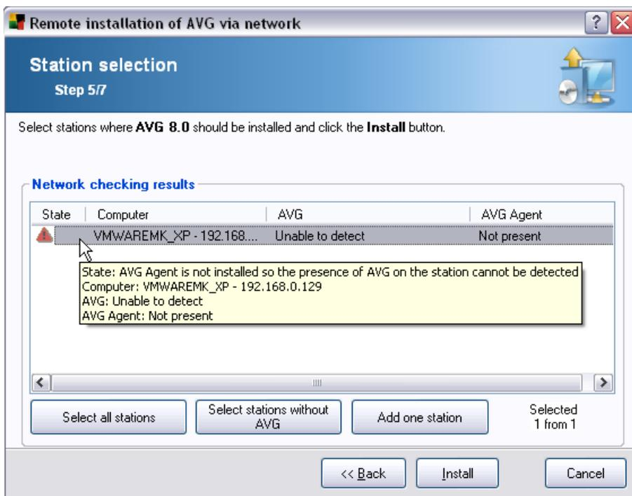
Additionally, you may display a so called 'tool tip' when pointing to a station in the list for a few seconds. The tool tip contains an overview of the station state and other details.
