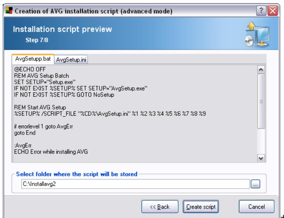
This step contains a preview of both setup and configuration files. The first tab contains information about the setup file and the second contains the presets.
