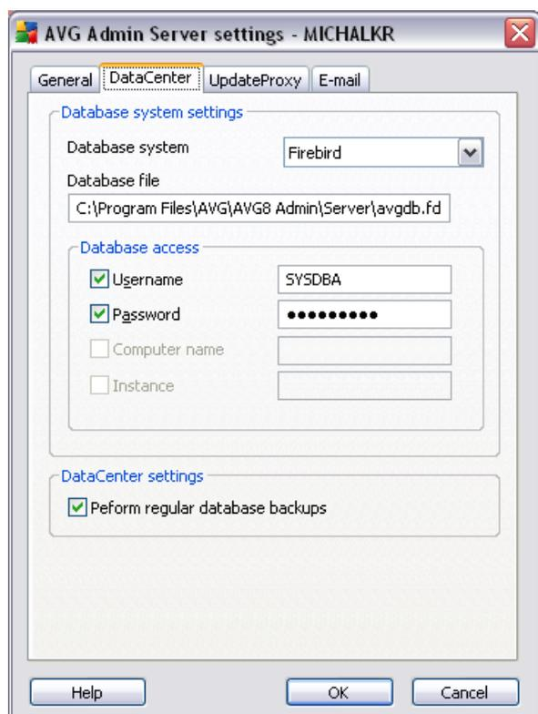
**Database system settings** section contains database options. To change the **database system**, choose a different one from the drop down list.
