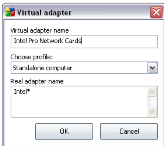
To the **Virtual adapter name** type in some preferred name of the virtual adapter. From the roll-down menu select the profile you wish to assign to this adapter. In the **Real adapter name** specify the name of the physical adapter available on the stations. You can use asterisk wildcard indicator (\*) to be used as a replacement for a part of the physical adapter name.
