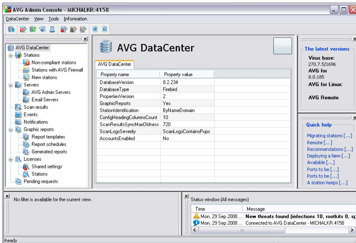
The **AVG Admin Console** interface is completely customizable allowing users to move or enable/disable individual panels according to their needs. Within the default view, all six panels are visible, in addition to a navigation toolbar and upper menu.
