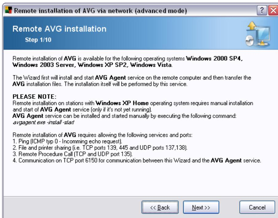
For correct remote installation, the wizard will first install and start the AVG Agent service on the target station, then transfer the AVG installation files and process the installation accordingly.
