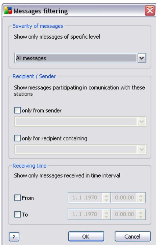
This option allows you to filter out messages according to more extensive parameters. From the drop down menu select what type of messages you wish to display.
