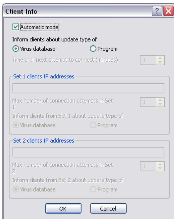
This dialogue is designed to set up the parameters of the update distribution from AVG Admin Server to clients, or between AVG Admin Servers. Two modes of update distribution are available – automatic and manual:
