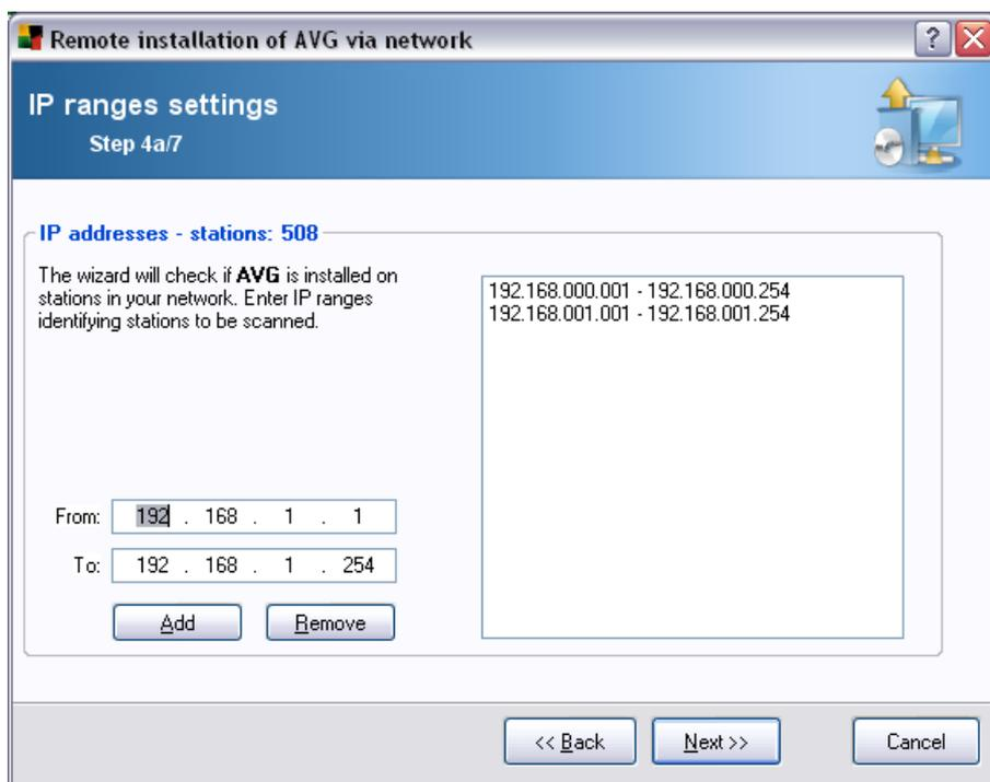
You need to specify the scanning range by entering the IP addresses here. In the **From** field enter a starting IP address and in the **To** field an ending address. Click the **Add** button to add the address into the list.
