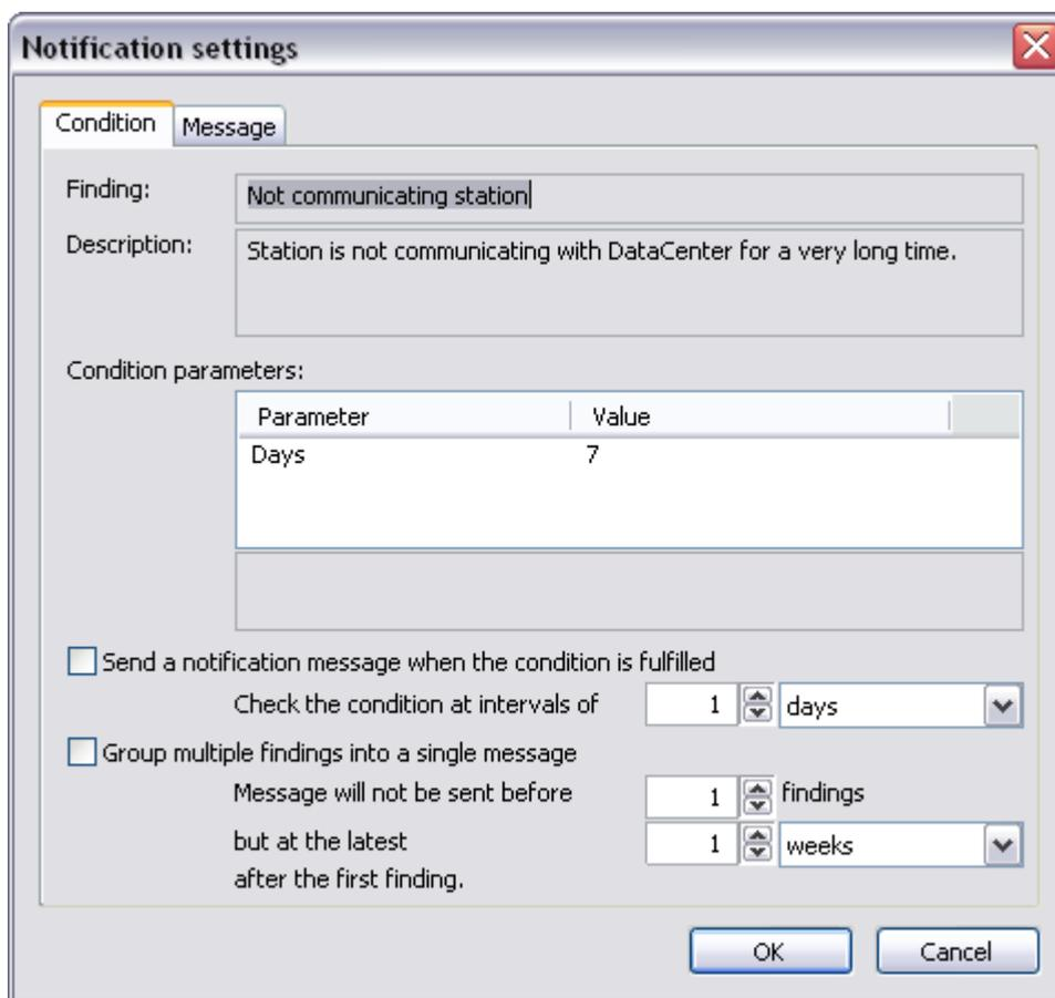
Check the ***Send a notification message when the condition is fulfilled***
