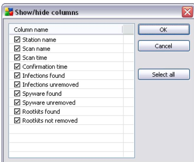
Here you can check or uncheck columns you wish to keep visible or hidden. Use **Select all** button to keep all columns visible.
